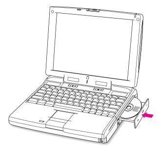
*Note:* When the CD-ROM drive is in use, you may notice some vibration as the compact disc spins rapidly. Certain discs can cause the drive to vibrate because they have heavily inked artwork or a label that creates an imbalance as the drive spins.
